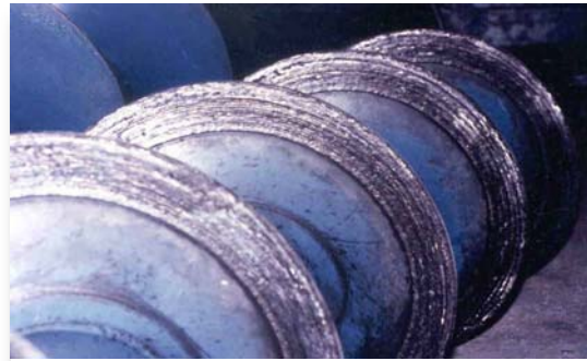
Screw Conveyor with Hardfacing
