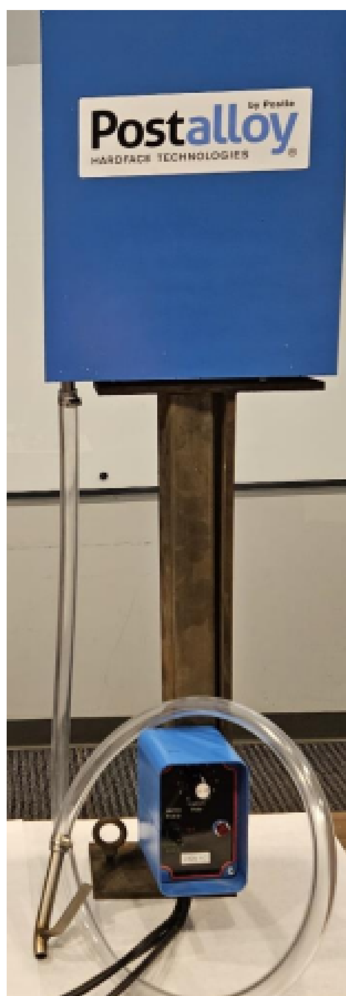
Figure 1: Typical setup for tungsten carbide drop
